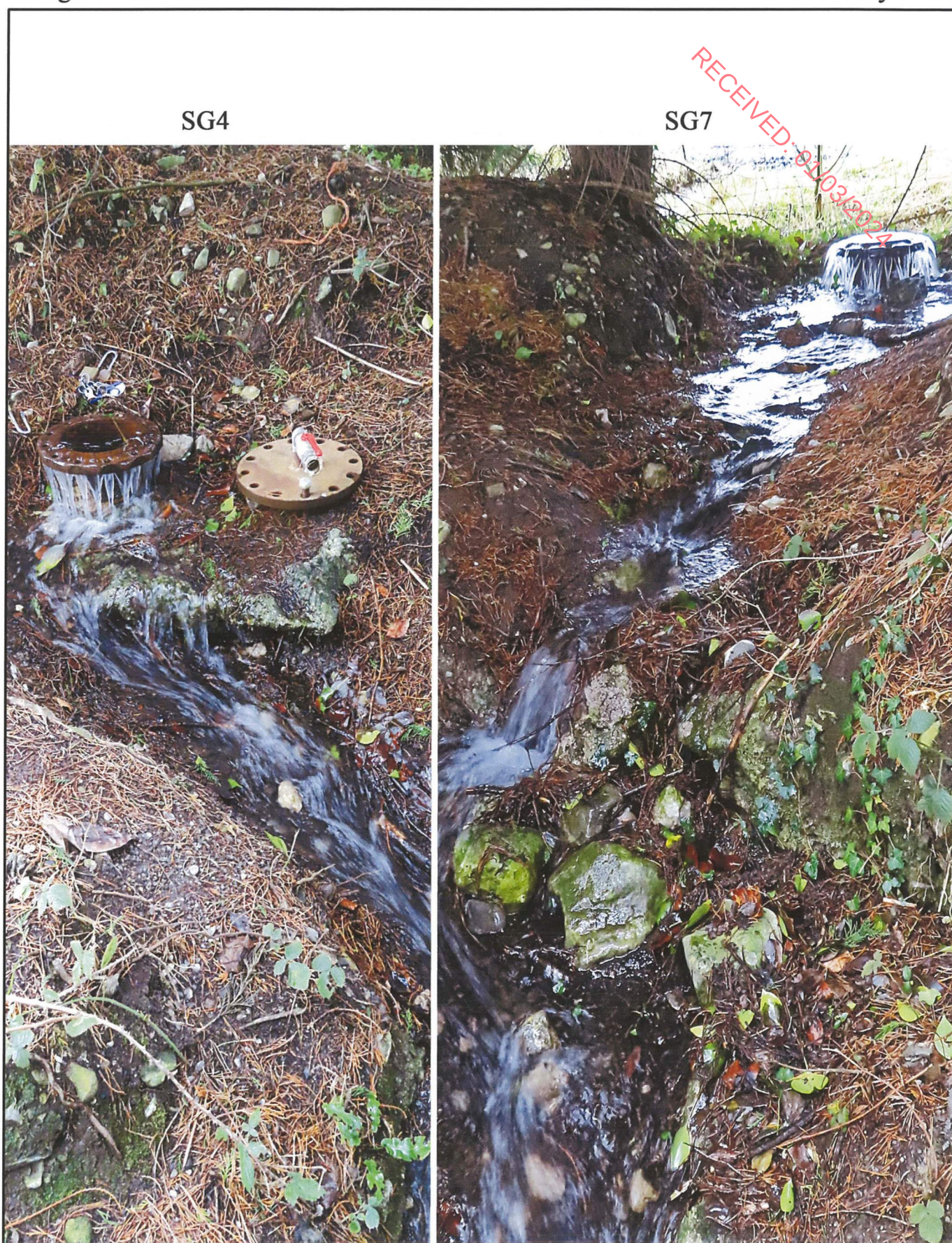
Figure 5.18 Artesian flow from Boreholes SG4 and SG7 on the 5th February 2021
